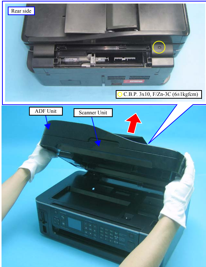
Figure 4-5. Removing the Scanner Unit/ADF Unit (2)
