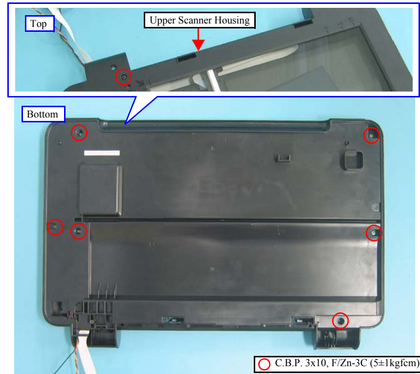
Figure 4-119. Removing the Upper Scanner Housing (1)
