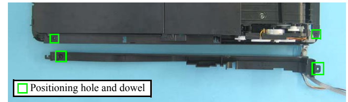
Figure 4-135. Installing the ADF Rear Cover
